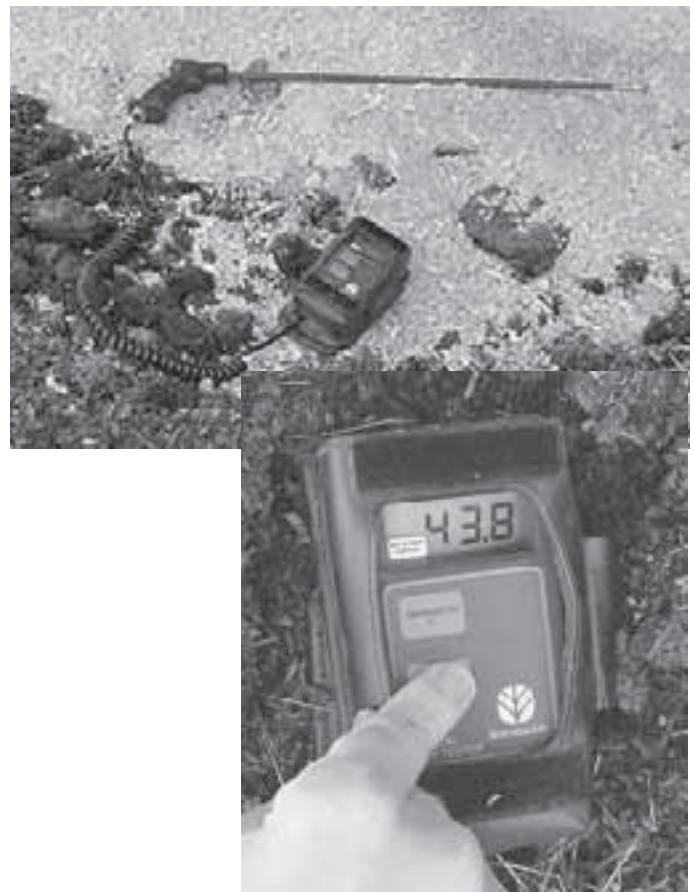
Figure 5: A hay moisture probe with a long stem works well to measure the moisture content of a compost pile. This pile is at the correct moisture level of about 45 per cent.
